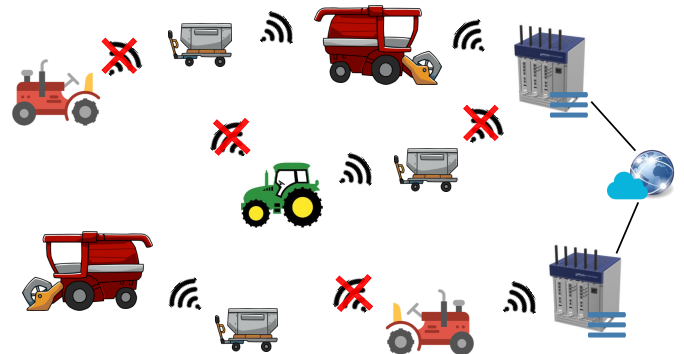
Fig. 1: Example of a dynamically evolving Wireless Mesh Network connecting multiple construction devices.
