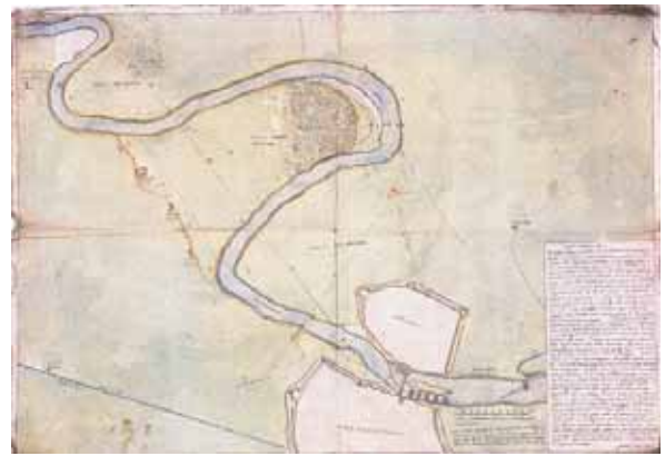
Fig. 3- Design for straightening of a tract of the Tanaro close to the city, signed by Clarici and drafted in 1593
