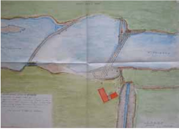
Fig. 1- Design by civil engineer Giovanni Battista Clarici, dated 1590, related to the lock on the Bormida River conveying the waters to the ancient Bettale canal
