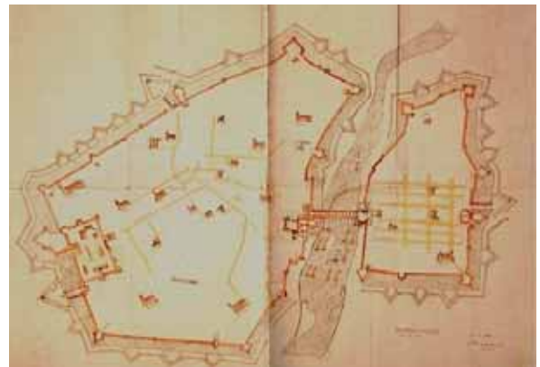
Fig. 6- Use of waterways for the defence of the urban environment in a planimetry study by Giovanni Pietro Pelucco, drafted in 1625 the last tract of the old river bed: in fact, the canal began in the area named la Valletta – about 7 miles from Alessandria – close to Gamalero, crossed the latter, dropped to Borgoratto and Cantalupo, reached the city by flanking the road named Bià or Betale. The tract starting about 3 miles away from the city was completely renewed. The proof of such – as described by Giacomo De Giorgi – are certain stone and wood remains that could still be found in the
