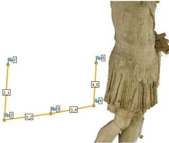
Figure 56. In order to scale the model, the distances between the targets have been measured and then used as scale bars in Photoscan
