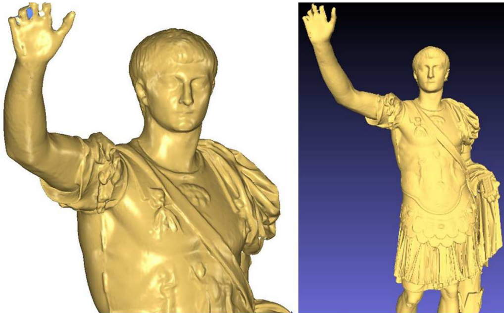
Figure 88. The mesh created with 3D Reshaper. Generation with the two steps tool: the user sets the mean triangles dimension and, in a further step, the deviation error in order to refine the final mesh.
