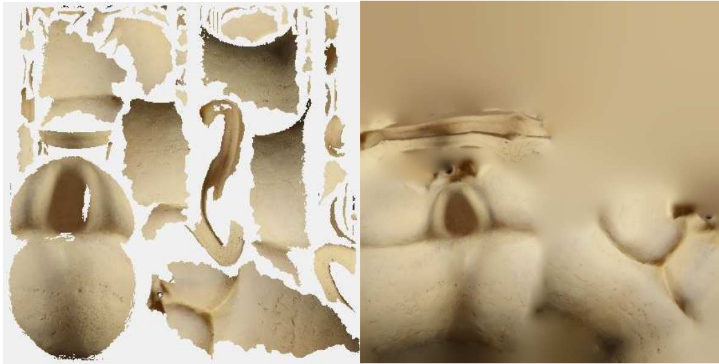
Figure 76. Left: automatically generated diffuse color map; right: new diffuse color map keeping the UV map edited in Blender.
