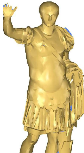
Figure 92. Ultra decimated Low Polygon (LP) surface - 7000 faces.
