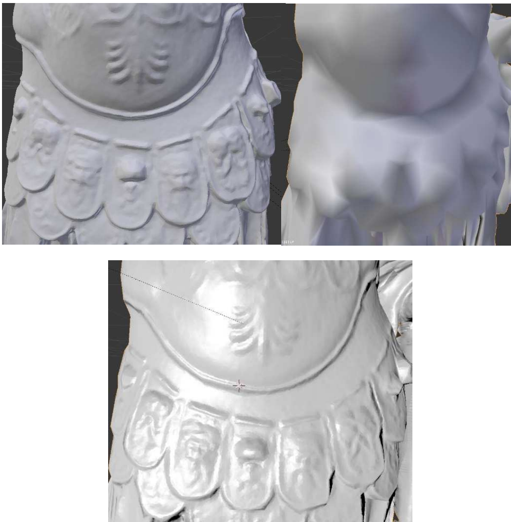
Figure 101. Visual comparison between HP model (above-left), LP one (above - right) and the same LP model with NM applied (below).
