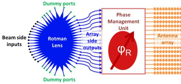
Fig. 2. Extended scan range concept block diagram
