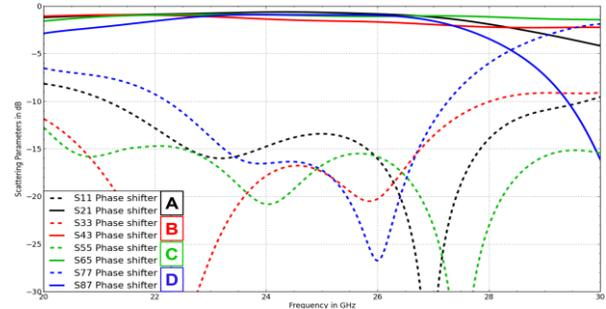
Fig. 4. Simulated *S*-parameters of the 4 reflective type phase shifters providing 90° (black), 180° (red), 270° (green) and 360° (blue).
