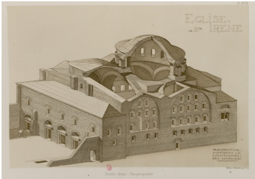
Figure 1: Perspective drawing of Hagia Irene Church showing the construction of the dome of the church. In Jean Ebersolt, Adolphe Thiers, Les Eglises de Constantinople , Paris, Ministère de L'Instruction Publique et des Beaux-Arts, 1910. This publication presents a restitutive survey of Byzantine churches in Constantinople with architectural drawings.
