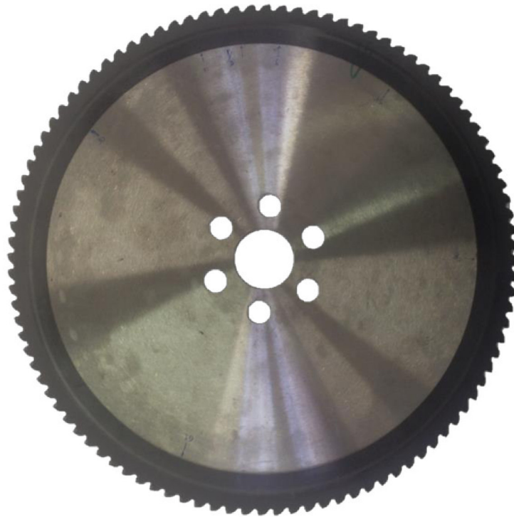
Figure 2. Coated TCT sawblade for cutting metallic alloys.
