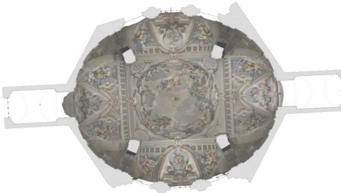
Figure 21. The orthophoto reproducing the vaults was generated by digital photogrammetry – sfm image processing.
