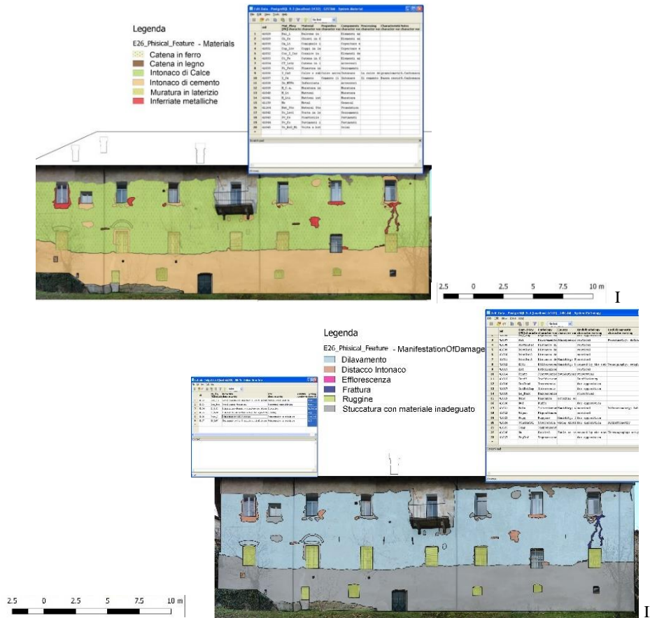
Figure 52. (I) GIS representation of the ‘Materials’ values mapped on the façade and related table in PgAdminIII. When possible, taxonomy values are used, preferably kept from the NORMAL documents; otherwise, other affirmed bibliographic sources were used (Carbonara, 2004). (II) GIS representation of the “ManifestationOfDamage” values mapped on the façade and related tables (Cerutti et al., 2015).
