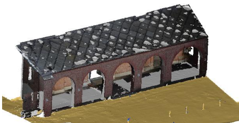
Figure 114. Only the narthex is visualized (LOS 2). Here, the model of the terrain is also visible and could be included in the CityGML model.
