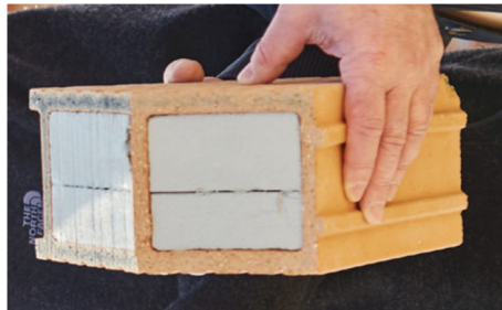
Figure 8: Fumed silica integrated brick [30]
