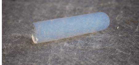
Figure 9: Solid aerogel placed upon an aerogel blanket [45]
