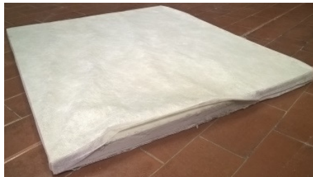
Figure 5: Fumed silica pressed board
