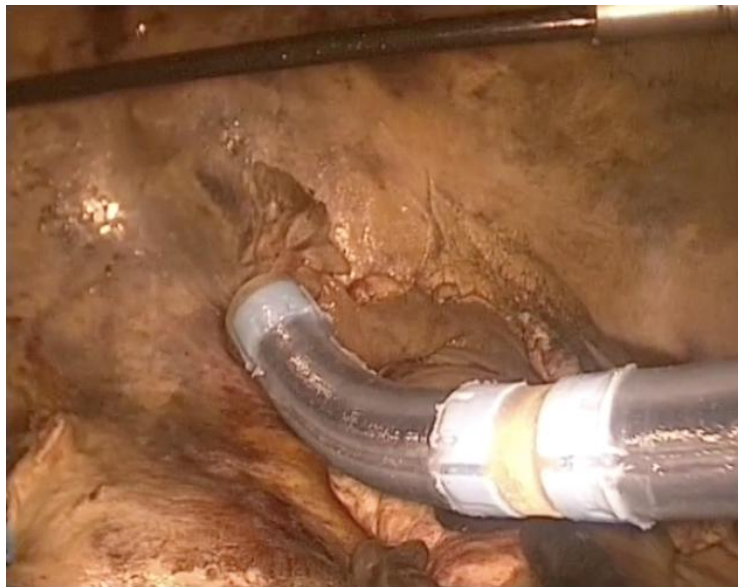
Figure 18 Overview of the embalmed abdomed using a 30° laparoscopic camera. The STIFF-FLOP arm was introduced and placed under direct vision
