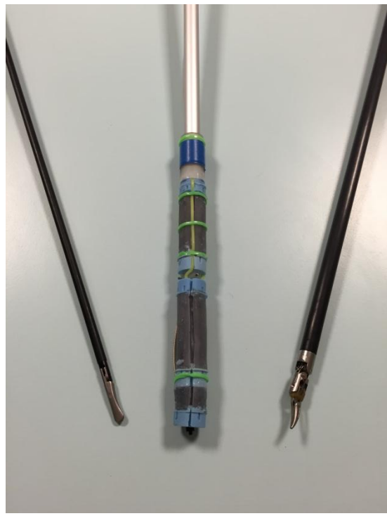
Figure 16 The thinner prototype (14.3 mm in diameter) compared to standard laparoscopic instruments
