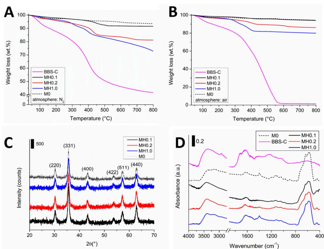
**Figure 1.** Physicochemical characterization of hybrid magnetic nanoparticles (HMNPs) and reference materials (BBS-C and M0): (A) thermo-gravimetric analysis (TGA) under nitrogen atmosphere, (B) TGA under air atmosphere; (C) X-ray diffraction (XRD) pattern of HMNPs (main reflections are labeled), and (D) absorbance FTIR spectra in transmission mode. Legend: M0 (black dotted line), BBS-C (magenta solid line), MH0.1 (black solid line), MH0.2 (red solid line), and MH1.0 (blue solid line).
