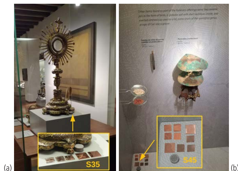
Fig. 3 – Sensors and Cu reference samples positioning in the National Museum of Colombia. (a) sensor S35 located in room 13; (b) sensor S45 located in room 6.
