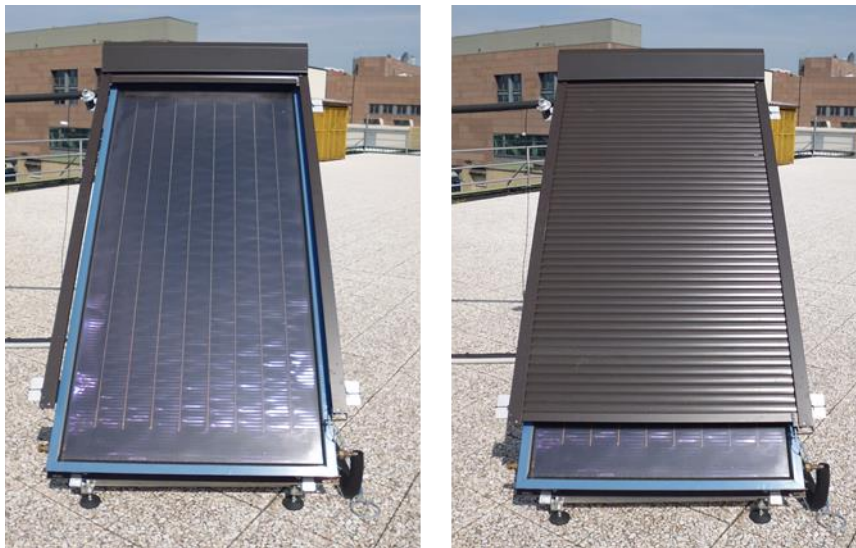
Figure 29. The solar thermal collector used in the full-scale prototype.
