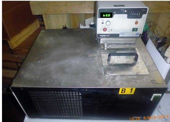
Figure 4. The thermostatic bath used to heat up to 60 °C the samples.
