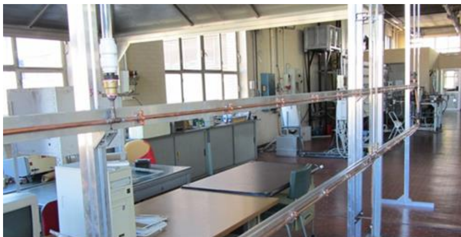
Figure 10. The pressure drops testing circuit.
