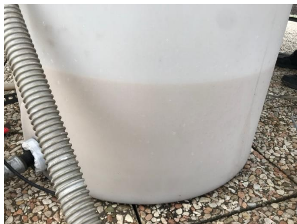
Figure 28. The version 2 of the thermal energy storage unit filled with mPCM slurry.
