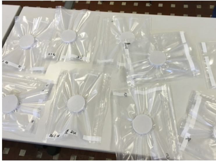
Fig. 3.2 Final packaging of the LiH pellets, made by UNITO. PE is surrounding the LiH to prevent contact with moisture present in water
