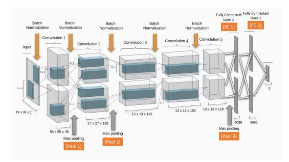
Fig. 4.5 AlexNet-BN Architecture
