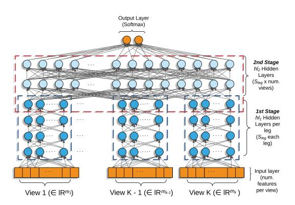
Fig. 3.4 *Spidernet* architecture. In the first stage, each view is independently processed by a network "leg" and projected into a common latent space. In the second stage, the transformed views are first combined and then classified.
