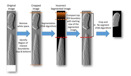
Fig. 4.3 An example showing the segmentation algorithm applied to Swipe 2013 images.
