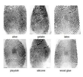
Fig. 2.2 Examples of live and fake samples (created with different materials) from the LivDet 2011 datasets.
