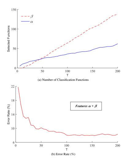
Fig. 3.3 (a) number of classification functions per view at each iteration and (b) behavior of the classification error in a two-view experiment for increasing values of T.
