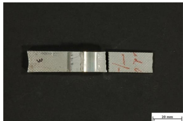
Figure 8. The tensile test result of \text{SiC}_p/\text{Al} MMCs joint.
