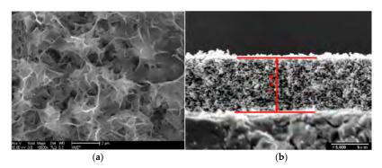
**Figure 7.** Examples of porous ZnO morphologies obtained by sol-gel methods. (**a**): a typical FESEM image of ZnO thin solid films deposited via a modified chemical bath deposition method. Scale bar is 2 μm. Reproduced with permission from [106]; Copyright 2006 Elsevier. (**b**): Cross-section FESEM image of ZnO films prepared at 0.05 mol/L methanolic zinc acetate solution and sintered at 500 °C. Scale bar is 5 μm. Reproduced with permission from [107]; Copyright 2005 Elsevier.
