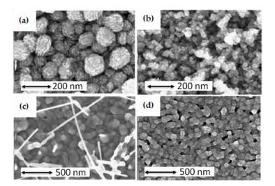
**Figure 2.** Surface morphologies of Zn films deposited on glass substrates with magnetron sputtering: (a) Ar, 2 mTorr; and (b) Ar +  $O_2$ , 2 mTorr. Surface morphology of ZnO films formed by thermal oxidation of Zn films at 600 °C in air for 1 h: (c) deposited in Ar, 10 mTorr; and (d) deposited in Ar +  $O_2$ , 10 mTorr. Adapted with permission from [35]; Copyright 2005 Elsevier.
