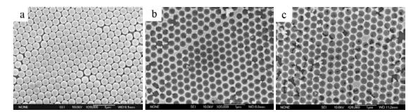
**Figure 8.** (**a**) A typical SEM image of the original PS opal templates. (**b**,**c**) SEM images of the 2D ordered ZnO porous films at different deposition times of (**a**) 40 min and (**b**) 2 h. Adapted with permission from [113]; Copyright 2005 Elsevier.
