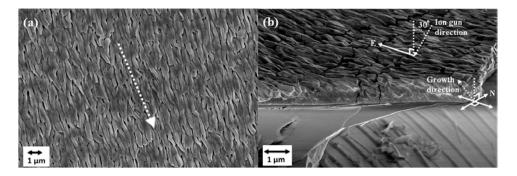
**Figure 1.** Scanning Electron Microscope low-magnification images: (**a**) Top view of as-synthesized ZnO film on glass substructure, where the white arrow indicates the projection of the incident flux on the film; (**b**) Cross-sectional view of the sample, where the ion flux and growth direction are denoted. Adapted with permission from [33]; Copyright 2013 Elsevier.
