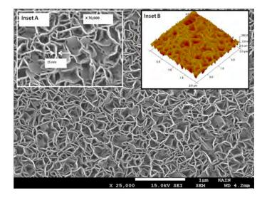
**Figure 4.** Low-magnification scanning electron microscope image and atomic force microscope profile of the 3D ZnO nanowall network grown vertically on Si(100) at 550 °C under 0.5 Torr O<sub>2</sub> background pressure. Scale bar is 1  $\mu$ m. Reproduced with permission from [51]; Copyright 2015 Elsevier.
