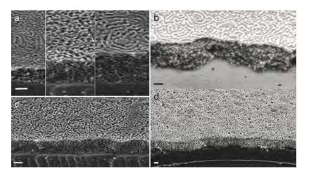
**Figure 10.** SEM of ZnO replication of the worm-like morphology: (**a**,**c**) worm-like PS template; (**b**) as-deposited ZnO-PS hybrid; (**d**) ZnO morphology after annealing at 400 °C followed by etching of the top compact layer. Scale bar are 200 nm. Reproduced with permission from [124]; Copyright 2014 John Wiley & Sons, Inc.
