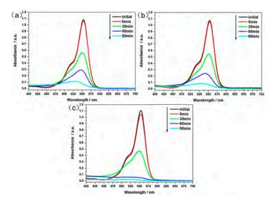
**Figure 6.** Absorbance spectra of Rhodamine-β dye aqueous solutions under UV irradiation, in presence of ZnO nanorod arrays (ZNRAs), synthesized for different electrodeposition times: (**a**) one time; (**b**) three times; and (**c**) six times. Reproduced with permission from [97]; Copyright 2014 Elsevier.
