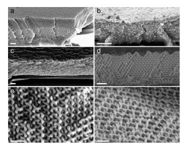
**Figure 9.** Side-view SEM images at a 45° angle of gyroid replication into ZnO: (**a**) gyroid PS template; (**b**) as-deposited ZnO-PS hybrid; (**c**) ZnO gyroid after annealing at 550 °C; (**d**–**f**) different faces of the ZnO gyroid shown in (**c**). Scale bars are 1  $\mu$ m for panels (**a**,**b**), 400 nm for (**c**,**d**), 200 nm for (**e**,**f**). Reproduced with permission from [124]; Copyright 2014 John Wiley & Sons, Inc.
