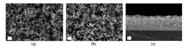
**Figure 3.** Field Emission Scanning Electron Microscope images of porous Zn thin films: (**a**) as-prepared; (**b**,**c**) after conversion into ZnO by thermal oxidation. Scale bar for (**a**) and (**b**) is 400 nm, for (**c**) is 2  $\mu$ m.
