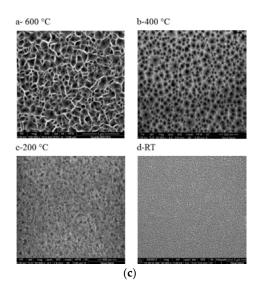
**Figure 5.** Scanning Electron Microscope images showing the effect of (**a**) deposition time, (**b**) oxygen pressure, and (**c**) substrate temperature on the morphology of the resulting ZnO nanowall network. Adapted with permission from [52]; Copyright 2014 Elsevier.
