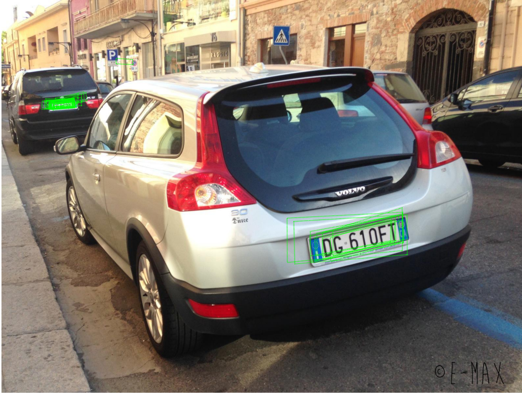
Fig. 5.2 Example of classification output of the fully convolutional plate classifier. Only localizations where the plate classification confidence is larger than 0.5 are shown.
