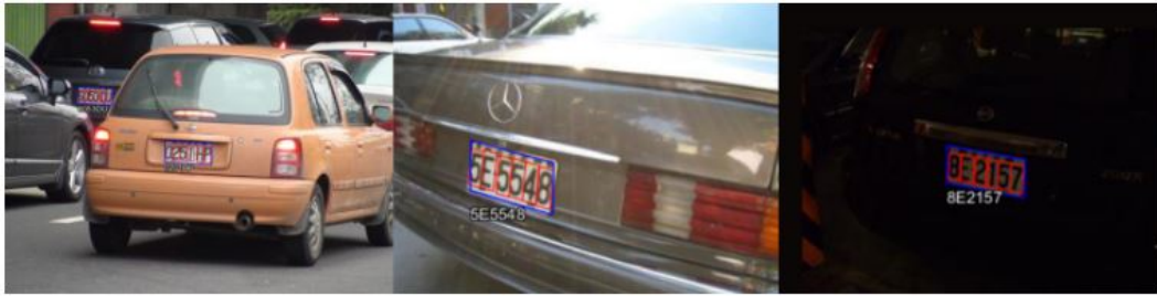
Fig. 6.13 Examples of AOLP images processed by our LPR system. Blue boxes correspond to detected plates, red boxes to detected characters (textual reading is superimposed).
