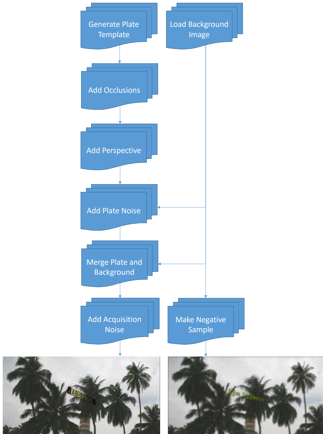
Fig. 3.1 Flow Chart of the sample generation algorithm. Each block is detailed in their corresponding sections.
