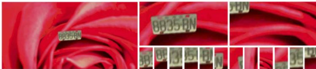
Fig. 6.12 Taiwanese synthetic training image (left) with corresponding plate training crops (positive: top center, negative: top right) and character training crops (positive: bottom center, negative: bottom right).
