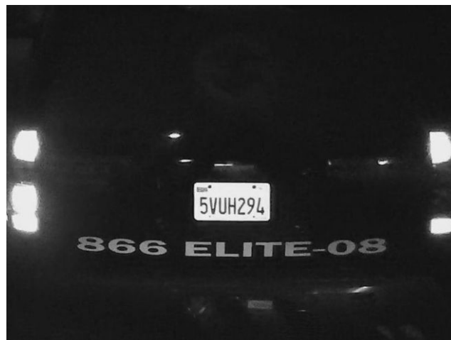
Fig. 1.1 Example of image acquired with dedicated hardware for license plate acquisition, including IR illuminator and IR pass filter on the camera combined with task customized shutter speed and aperture settings. Downloaded from: http://elitevirtualecurity.com/cctv-systems
