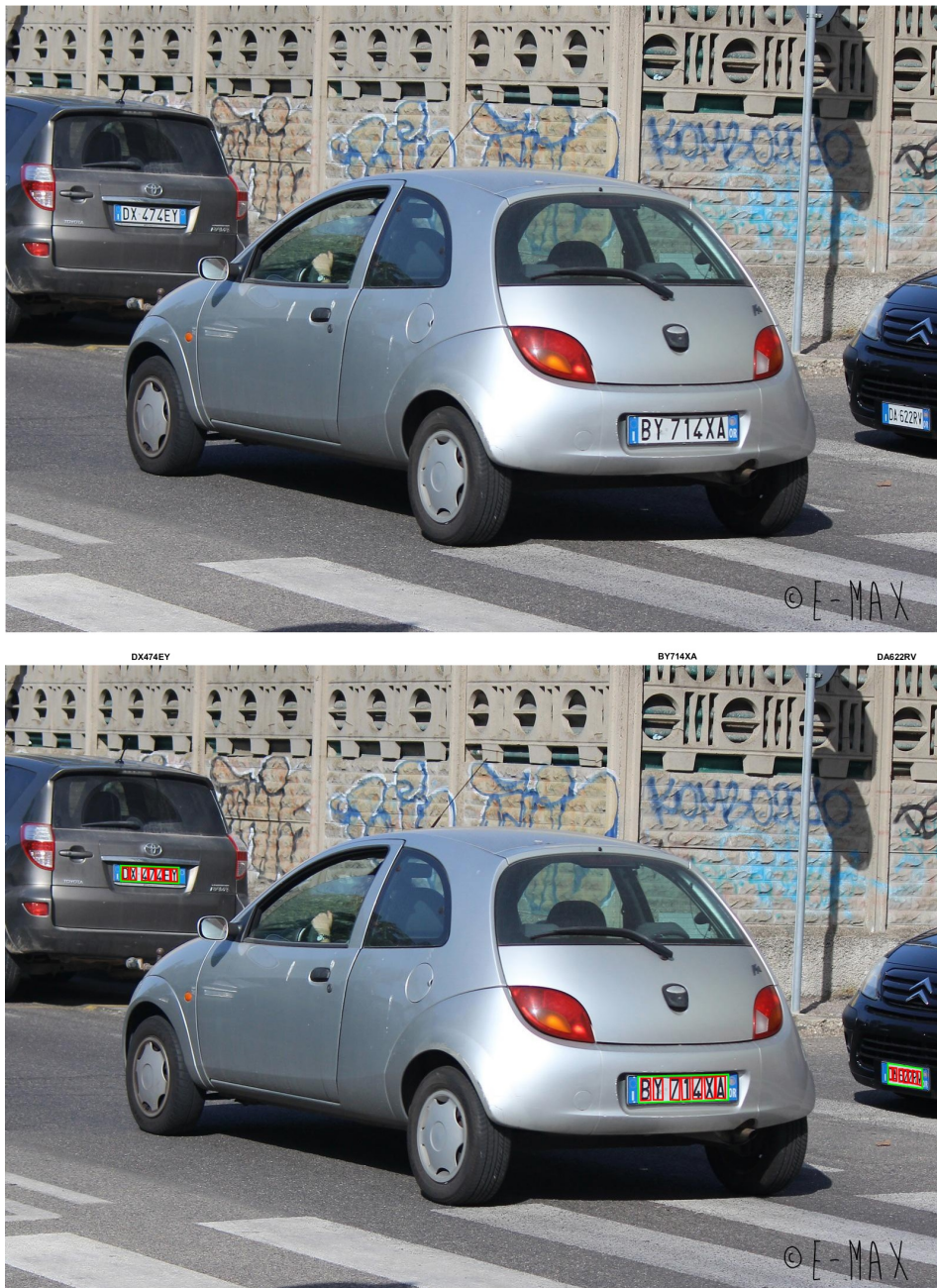
Fig. 5.5 Example of output classification of an image with multiple cars, license plate readings are placed above the image for readability.
