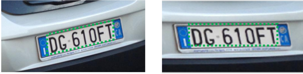
Fig. 5.3 Example of the rectification of a plate based on the refined corners localizations from section 5.4. As can be seen, if the horizontal difference between the of the corners on each side is not bad, the horizontal orientation of the plate will be corrected, but it will appear skewed.
