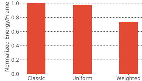
Fig. 4: Energy due to MAC operations for classifying one frame in LeNet-5.
