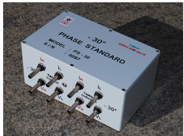
Figure 6. Schematic (a) of the negative phase standards and photograph (b) of the 0097 standard. The box in figure (b) contains two phase standards: in this paper, the standard on the left is identified with the suffix “A”; the one on the right, with the suffix “B”. The sockets labelled Temp. Control and Temp. Indicator are connected to two thermistors sensing the box temperature, one for the external temperature controller and one for the operator.
