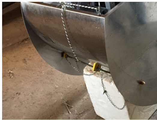
Fig. 4.6 1:45 PeWEC scale device mooring connection system.
