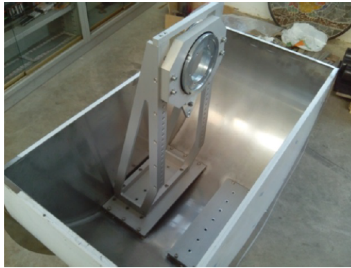
Fig. 4.7 1:45 PeWEC scale floater with frame installed inside.
