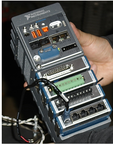
Fig. 4.13 NI CompactRio and its modules during the installation into the prototype.
