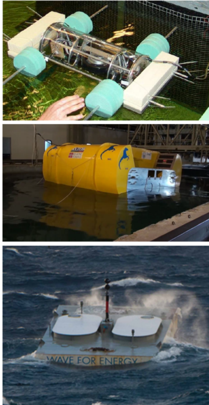
Fig. 2.5 ISWEC 1:45 scale device (top), 1:8 scale prototype (middle) and full scale device (bottom).
