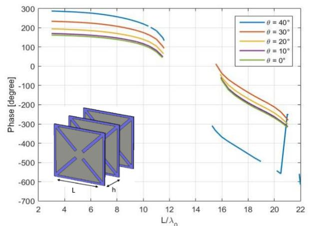
Fig. 1 - Malta-cross based unit-cell: variation of the  $S_{21}$  phase with  $L/\lambda_0$  computed for different angles of incidence. Inset: sketch of the unit-cell.
