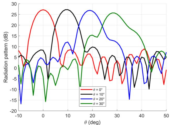
Fig. 6. Perforated dielectric TA: simulated radiation patterns in the E-plane for different angles of rotation of the feed.
