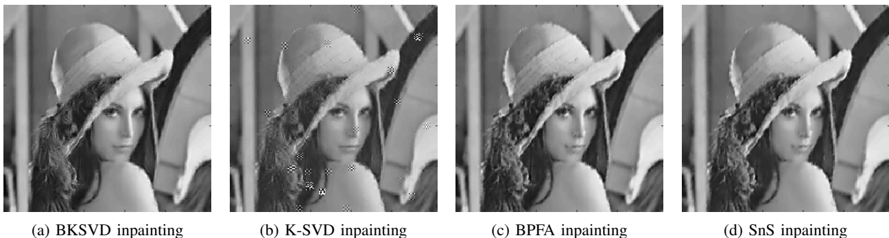
Fig. 5: Comparison of the inpainting performances at r = 75\% of BKSVD, K-SVD [60], BPFA [30] and Spike and Slab (SnS) model [35] algorithms. Please note that in this comparison the dictionary is learnt from the corrupted images themselves.
