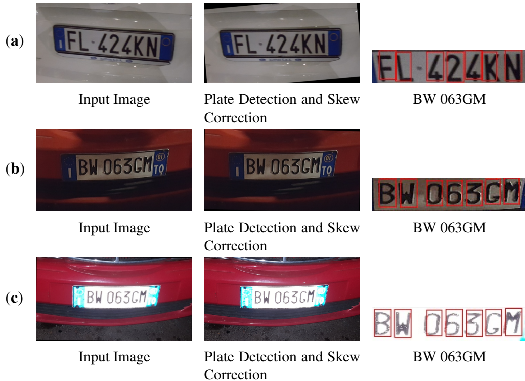
Fig. 6.5 Images captured at night in different imaging conditions: (a) image captured with perspective distortion; (b) image captured with insufficient illumination; (c) image captured with over-exposure and reflections due to speed-light.
