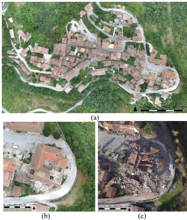
Figure 2. Digital orthoimage by UAV in Accumoli, flight height 130m (September 2016), GSD= 5cm/px. Comparison between T1-T4 in the eastern area of Accumoli: zoomed excerpt of T2, September (b) and T4, December (c).
