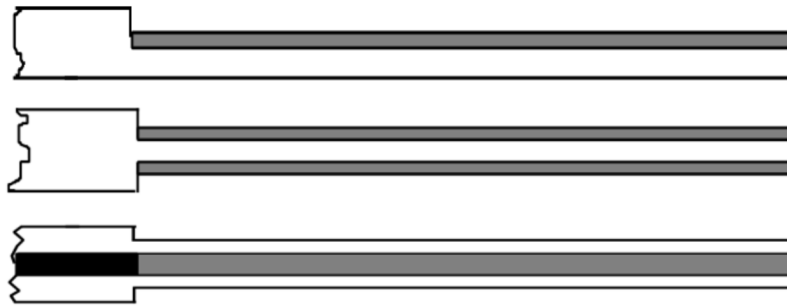
Figure 1 The Oberst beam configurations: single free layer (top), two free layers (centre), constrained layer (bottom). Grey colour indicates the damping material.
