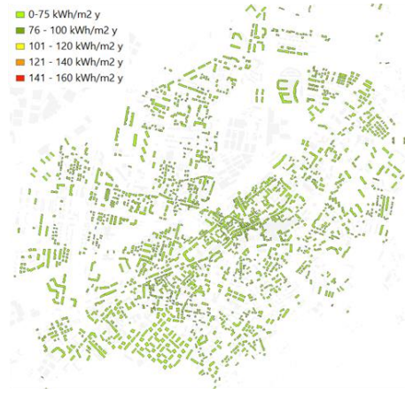
Figure 39: Heating demand Map following the Minergie-P renovation.
