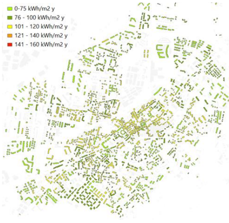
Figure 39: Heating demand Map following the Minergie-P renovation.
