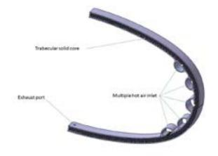
**Figure 1**: Schematic drawing of the panel integrated into the leading edge of wings.
