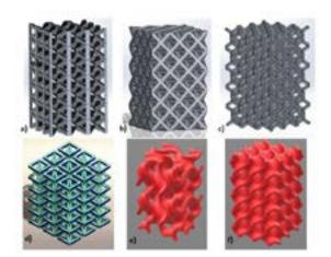
Figure 2: 3D models of specimens with different cell shapes: a) bccz, b) octet-truss, c) rombic dodecahedron, d) auxetic, e) Gyroid and f) schwarz diamond.
