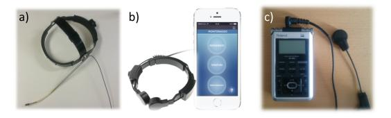
Fig. 6.12 The 3 devices used for acquiring the voice signal: a) the headset microphone (MIC); b) the piezoelectric microphone (PM) and c) the condenser microphone (ECM).
