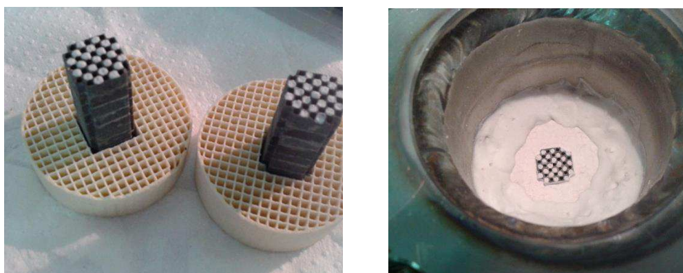
Figure 106 Small DPF are manually plugged and inserted into cordierite adaptors, to fit the mid-scale canning (128)
