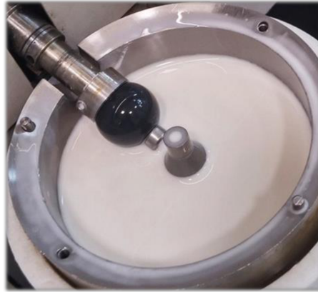
Figure 62 MTM pot, with mounted specimens, charged with 0,5% w h-BN PAO4, at the end of a test. It can be noticed the good wettability of the lubricant of the steel surface, maybe due to a less smooth surface than DLC.
