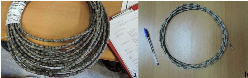
Figure 68: a) diamond wire employed for cutting stone benches or squaring blocks; b) diamond wire employed for producing slabs with multiwire machineries.
