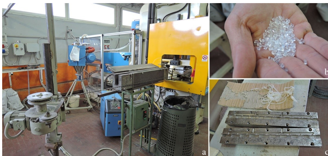
Figure 69: a) machinery for coating diamond wires; b) thermoplastic granules; c) mold employed for coating diamond wires with plastic.
