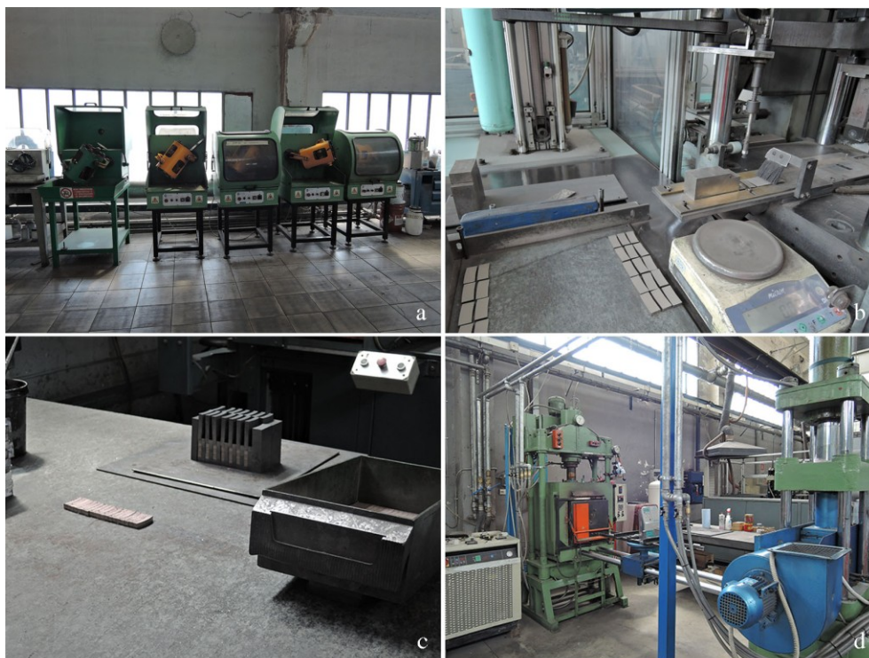
Figure 80: Production chain of diamond sectors: a) mixing of metallic and diamond powders; b) cold pressing of powders; c) preparation of green bodies to the sintering process; c) sintering of diamond sectors
