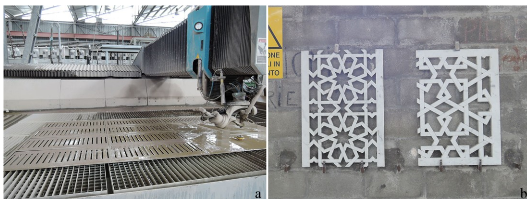
Figure 28: a) waterjet cutting machine; b) marble slabs cut with waterjet cutting technology
