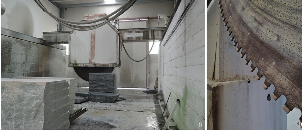
Figure 22: a) giant disk cutting a hard stone block; b) detail of a giant disk
