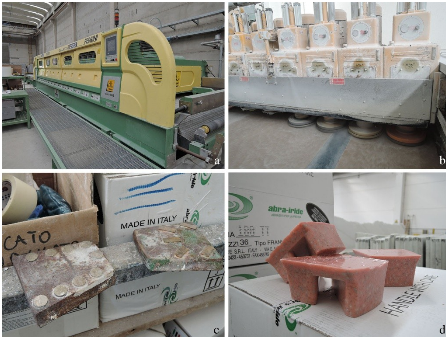
Figure 27: a-b) smoothing/polishing machines; c) metal abrasive for smoothing; d) diamond resin abrasive for polishing
