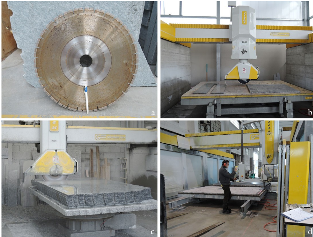
Figure 26: a) diamond disk; b-c) diamond disks with different diameters cutting stone strips (a) and slabs (b); d) worker programming the disk cutting machine
