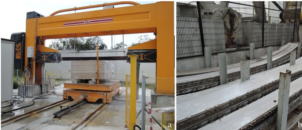
Figure 21: a) squaring of a marble block with mono diamond blade technology; b) worn out diamond blades
