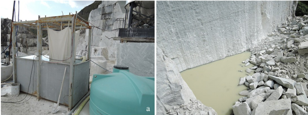
Figure 30: a) filter bag in a soft stone quarry; b) waste water from a hard stone quarry.
