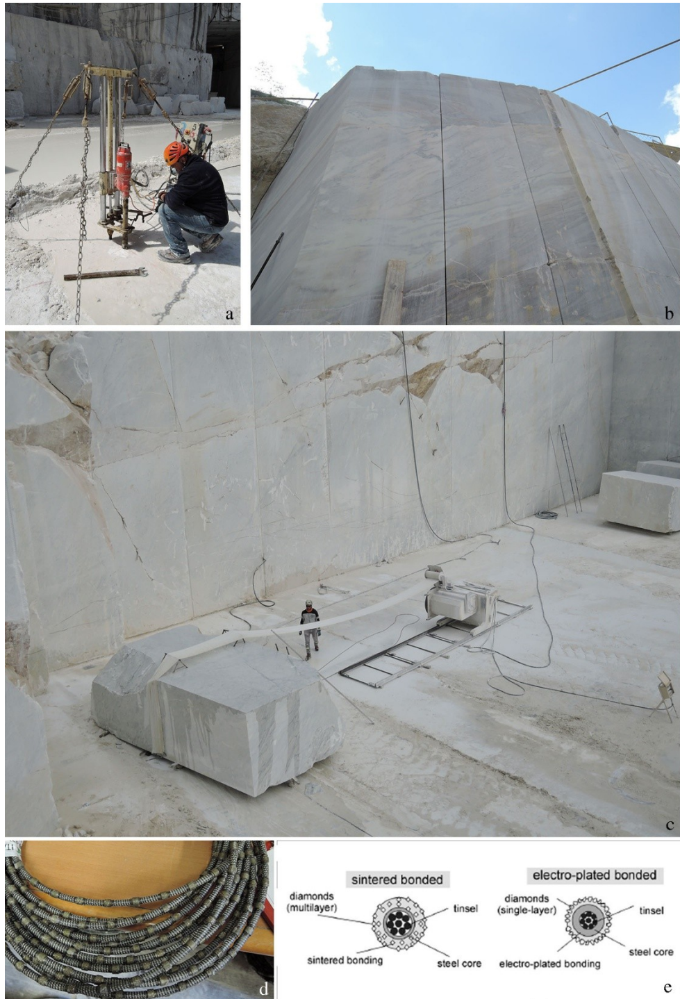
Figure 17: a) holes drilling ;b) marble bench with vertical cut made with diamond wire technology; c) quarryman preparing a block to be squared with diamond wire technology; a) electro-plated diamond wire; b) scheme summarizing the difference between sintered and electro-plated diamond beads (source: Tonshoff and Hillmann-Apmann, 2002)
