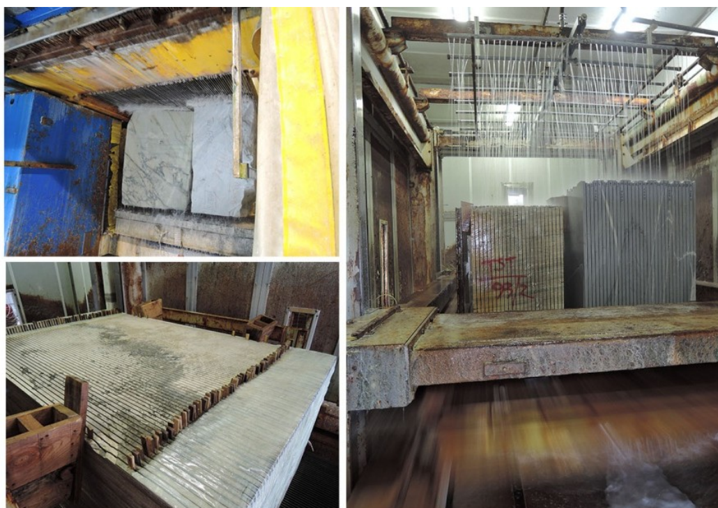
Figure 24: cutting of marble blocks with diamond multiblade saws technology
