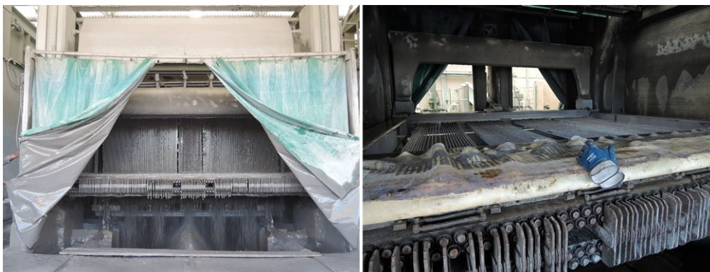
Figure 23: cutting of hard stone blocks with steel grid gang saw technology
