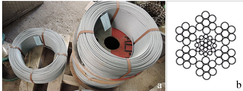
Figure 71: a) picture of the steel wire employed for the production of diamond wires employed in quarries; b) cross-sectional scheme of the steel wire.
