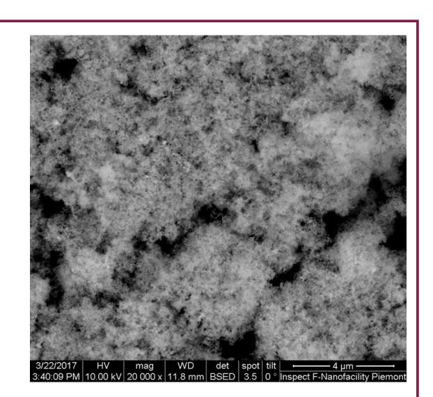
The fabrication procedure is schematically represented above. P25 TiO 2 paste 10% w/w in ethanol is prepared and homogenized in ultra-sonic bath at 15°C and at a power of 80 W to obtain stable and well de-agglomerated nanoparticles. A thin porous film on glass substrate is obtained using a glass stick as a rolling pin by manual Doctor blade deposition, with the help of a mask defining an area of 1 cm<sup>2</sup>
