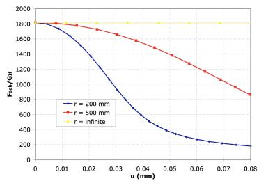
Figure 7. Load vs. loaded-end displacement during debonding.
