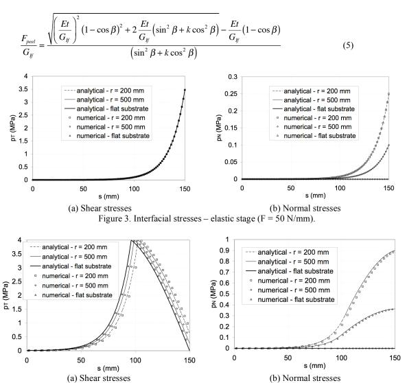
Figure 4. Interfacial stresses – elastic-softening stage at the initiation of debonding ( $F = F_{deb}$ ).
