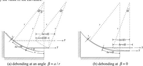
Figure 6. Schematics of the debonding process for a flexible but inestensible thin plate.
