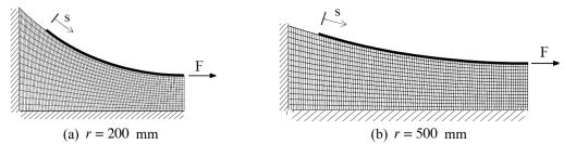
Figure 8. Mesh used in the numerical analyses.
