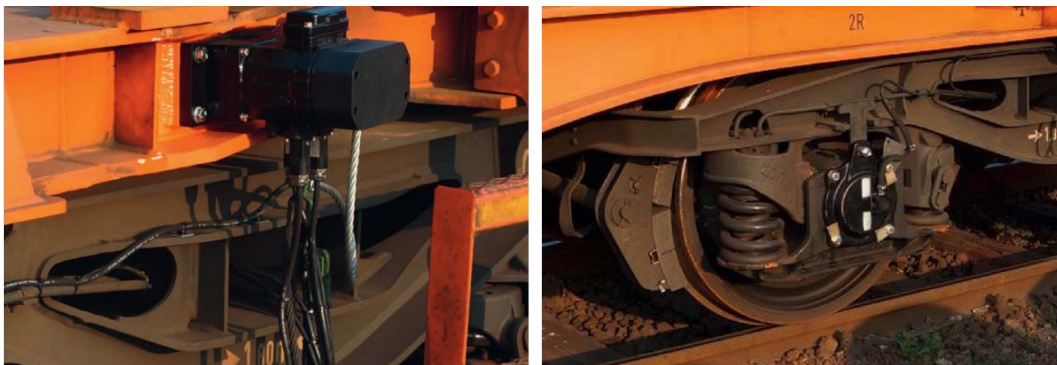
Figure 8. CargoCBM, on the left the OBU installed on a Wascosa wagon, on the right an axle box bearing sensorized.
