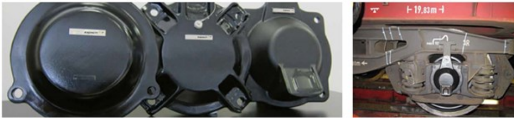
Figure 13. On the left different axle box cover for monitoring different axle box, on the right the monitoring system installed.
