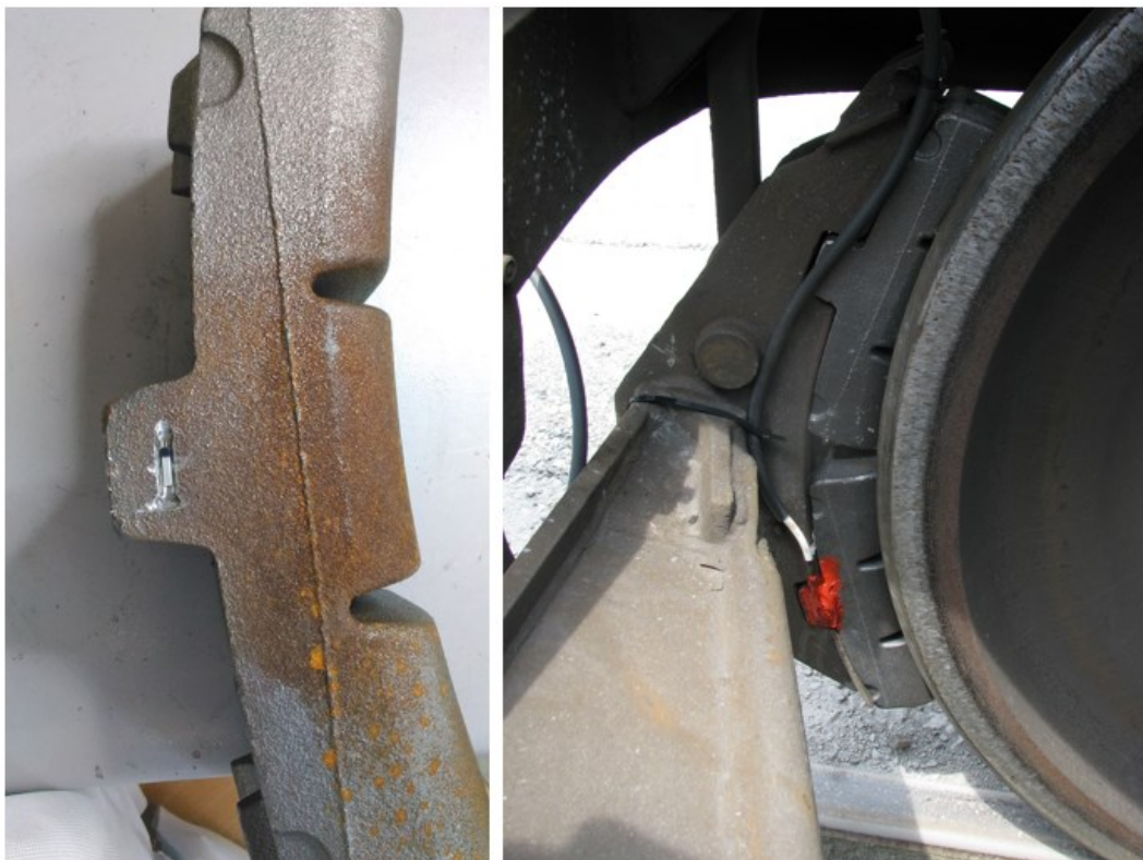
Figure 31. Brake block sensorization.
