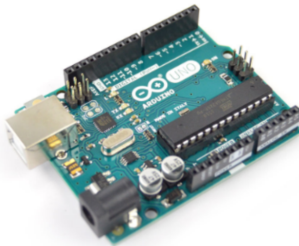
Figure 5.37 Arduino Uno R3 USB Microcontroller [139].
