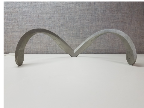
(a) Matlab Wiper model (front view). The blue line is the moving Wiper. The green line represents the static positive feature. (b) Stainless Steel 3D-printed Wiper (front view).
