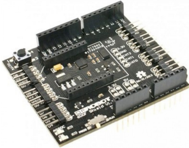
Figure 6.5 Inertial Mass Unit [143].
