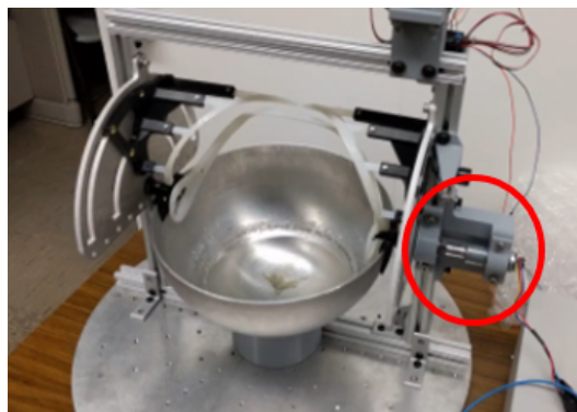
Figure 6.22 Water Wiper testbed with the Motor No.1 location (red circle).
