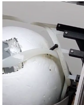
(c) Pin moves on the Wiper profile.
