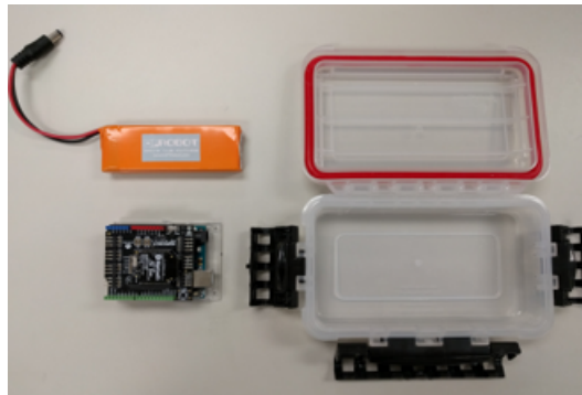
Figure 6.4 Water proof electronic box (open) [124].
