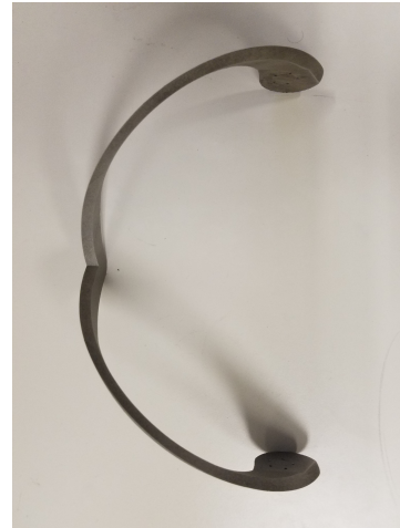
(a) Matlab Wiper model (top view). The blue line is the moving Wiper. The green line represents the static positive feature. (b) Stainless Steel 3D-printed Wiper (top view).
