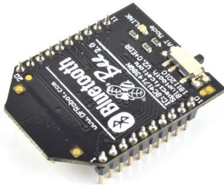
Figure 6.6 DFRobot Bluetooth Bee wireless module [143].
