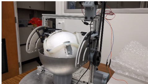
(c) Wiper engages with the pin and rotates the OS forward.
