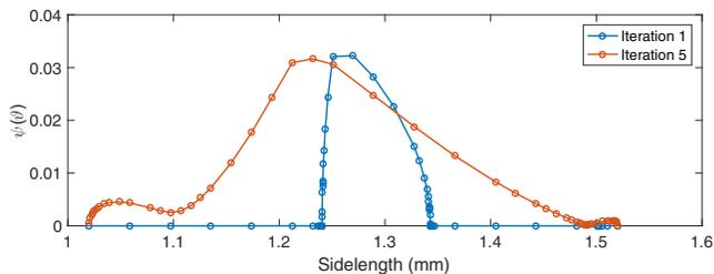
Fig. 3. Hamiltonian spectral distance  $\psi(\vartheta)$  from the imaginary axis, plotted for the initial model (Iteration 1) and the final model after passivity enforcement (Iteration 5). The final model is passive, since  $\psi(\vartheta) > 0$  for all  $\vartheta$  in its range.
