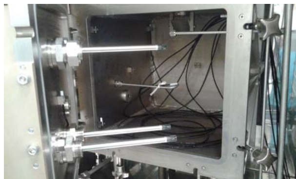
Fig. 10. Three Michell prototype sensors mounted inside the VSL chamber. Tests were carried out at temperatures up to 180 °C and pressures up to 550 kPa.
