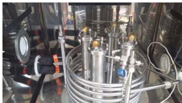
Fig. 8. Measurement chamber of the CETIAT humidity generator.
