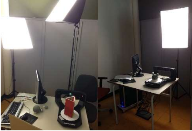
Figure 5. Different lighting setup, the best results are achieved with the set-up on the right
