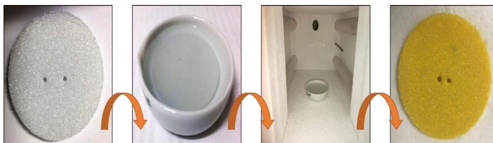
Fig. 7.1 impregnation method used for \beta - \text{Bi}_2\text{O}_3 deposition on sintered silica substrate
