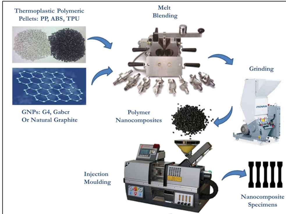
Figure 52 Schematic nanocomposites chart flow production
