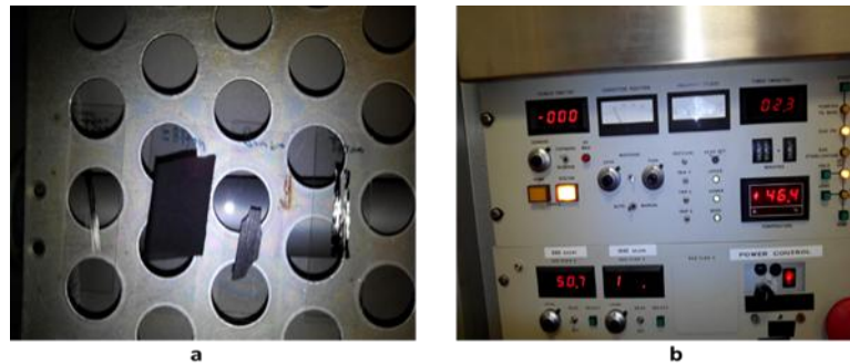
Figure4.4 : (a) Sample placement, (b) controls of Plasma Fab 508.
