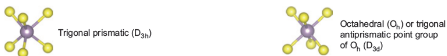
Figure 2. 39. metal coordination for layered TMDs. Atom colour code: purple, metal; yellow, chalcogen. 297
