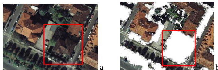
Figure 6: Portion of an aerial image (a) with a dark roof (red square) and the lack of relevant information in the generated point cloud (b).
