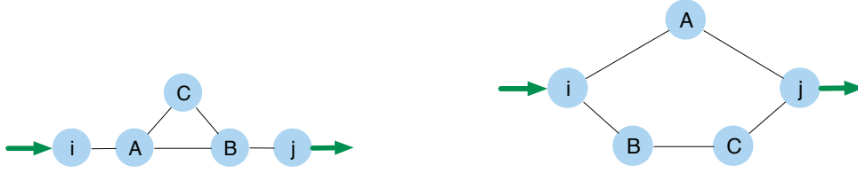
Figure 4.1: Toy examples illustrating the Shapley value computation. On the left graph, two acyclic paths exist between i and j , one augmenting the other. On the right graph, alternative paths exist between i and j . Dark arrows represent the traffic request from node i to node j .
