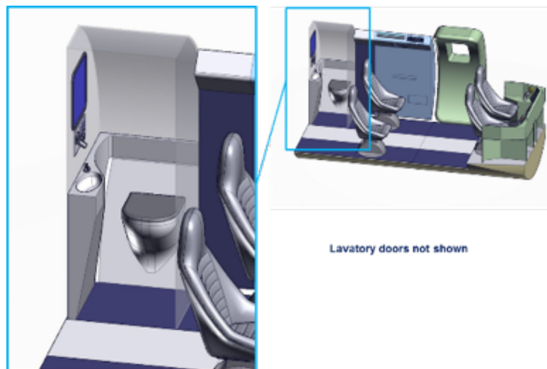
Figure 233: Lavatory design (left) and integration (right)
