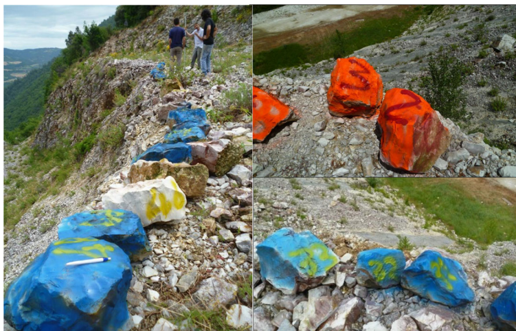
Fig. 3 Some of the blocks painted in bright colors and numbered, used for the man-induced rockfalls simulation
