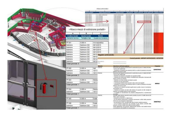
Figure 69: Extinguishing means inventory.
