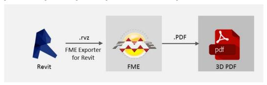
Figure 85: Revit-3D PDF interoperability process.
