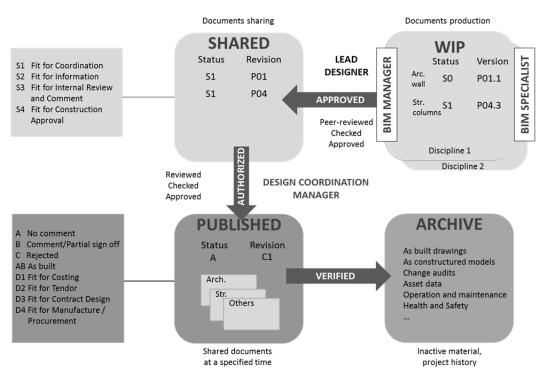
Figure 22: Common Data Environment description. Source: Re-elaboration of the BS 1192-2 scheme.
