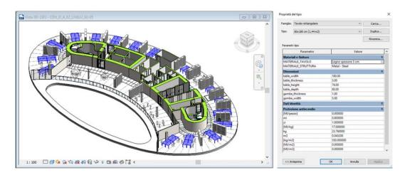
Figure 72: Desk parameters for specific fire load calculation.
