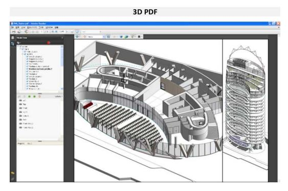
Figure 78: BIM model visualization through PDF 3D.
