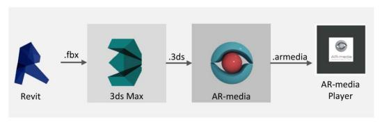
Figure 96: Revit-AR-media interoperability process for AR.
