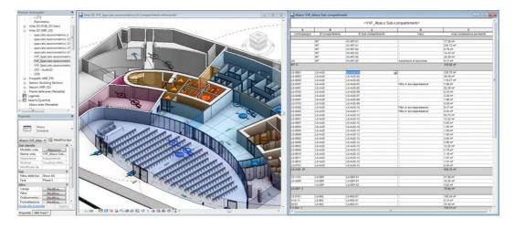
Figure 66: Fire compartments and systems installed schedule.
