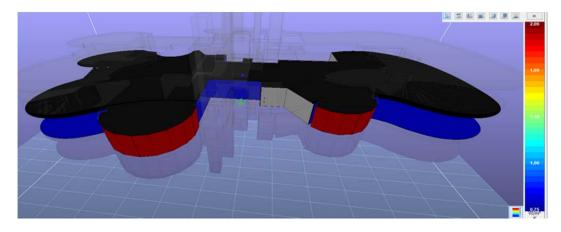
Figure 54: Visualization problems of curved walls in the EC770. EEB Project. Case study: Biblioteca Archimede, modeled by Maurizio Dellosta.
