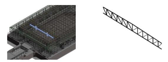
Figure 82: Rods in a reticular beam grouped by Assembly.
