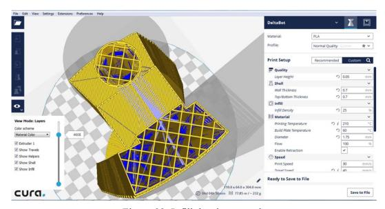
Figure 92: Infill density control.
