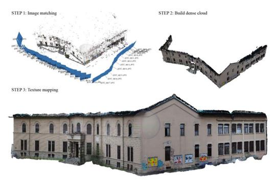
Figure 20: Point cloud realized with PhotoScan. TOBIM project. Case study: Corso Ferrucci 122.
