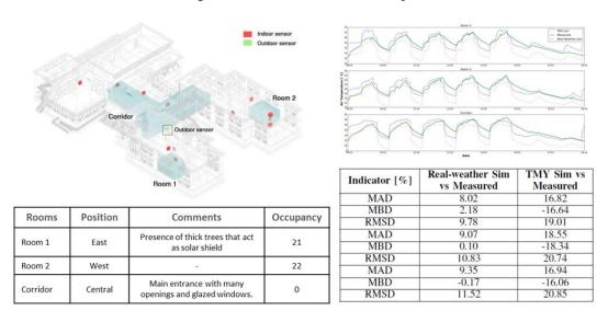
Figure 60: Simulated and measured indoor air temperature trends. EEB Project: Case study: Rodari school, modelled by Ossama Sabbar.
