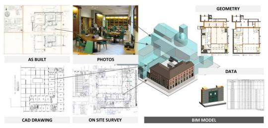
Figure 21: BIM model definition from survey and esisting documentation. TOBIM Project. Case study: Archivio Storico della Città di Torino, modelled by Aitana Marcos Guinea.
