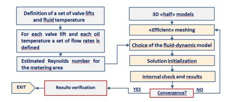
Figure 74: Procedure for the CFD survey
