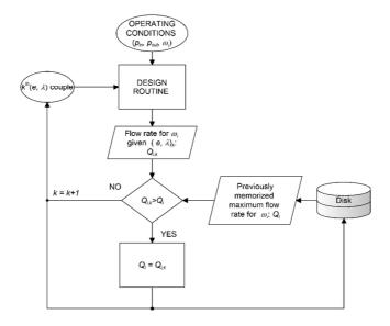
Figure 47: Routine to assess the maximum pump capacity conditions
