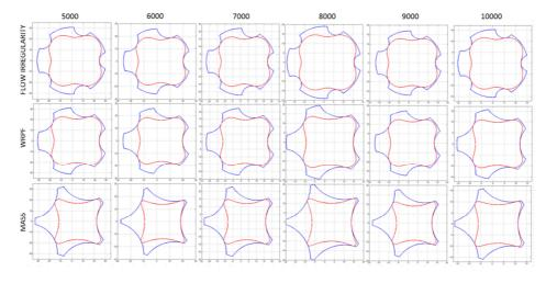
Figure 59: Optimized cycloidal profiles in the 5000 – 10000 rpm range
