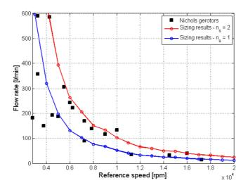
Figure 16: Simplified design tool: comparison with Nichols catalogue
