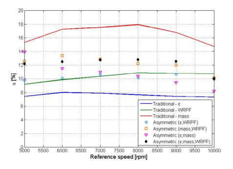
Figure 61: Multi objective optimization results: flow rate irregularity
