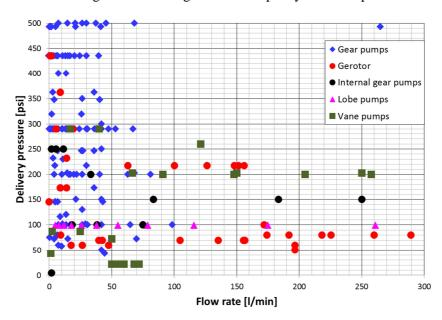
Figure 12: Catalogues data – delivery pressure vs flow rate
