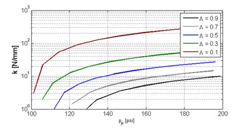
Figure 88: Required spring stiffness -  $45^{\circ}$
