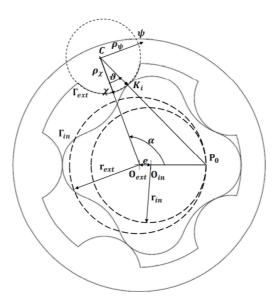
Figure 24: Geometrical parameters for gerotor profile definition
