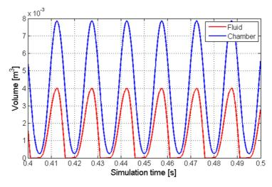
Figure 28: Effects of under sizing of the suction port
