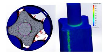
Figure 35: Rotors' mesh (left) – FEM result example (right)
