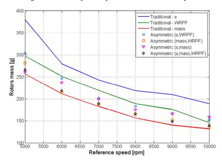
Figure 63: Multi objective optimization results: rotors mass
