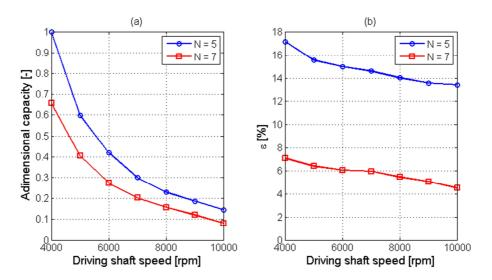
Figure 48: 5 vs 7 teeth gerotors: (a) displacement – (b) flow irregularity
