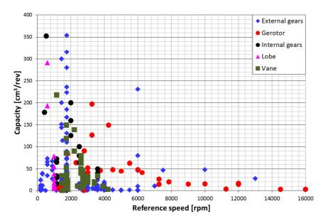
Figure 11: Catalogues data - capacity vs rated speed
