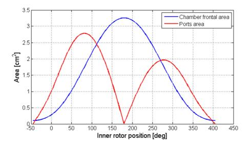
Figure 30: Ports vs chamber behavior (radial port configuration)
