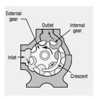
Figure 8: An internal gear pump with crescent<sup>3</sup>
