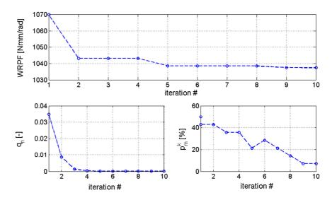
Figure 56: Algorithm behavior for n = 5000 rpm, WRPF optimization
