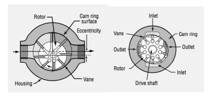
Figure 10: Unbalanced and balanced vane pumps<sup>5</sup>
