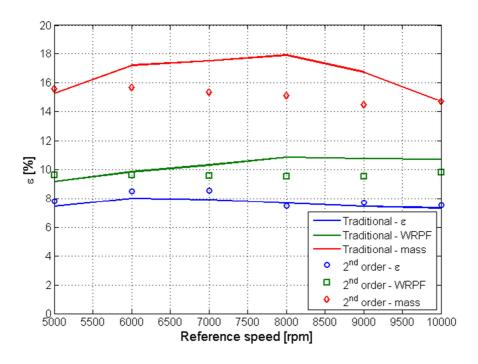
Figure 65: 2<sup>nd</sup> order optimization results: flow rate irregularity
