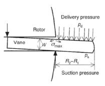
Figure 19: Simplified theory for vanes structural behavior
