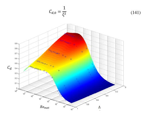
Figure 79: Polynomial fitting vs CFD results,  $\alpha = 45^{\circ}$
