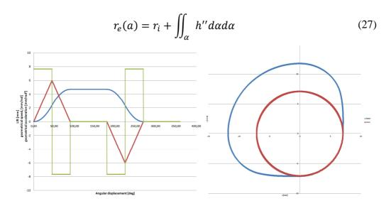
Figure 18: Example of motion law for the vanes lift and resulting geometry
