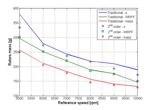
Figure 67: 2<sup>nd</sup> order optimization results: estimated rotors mass
