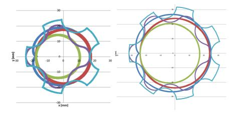
Figure 15: Examples of gerotor profiles (simplified design tool)
