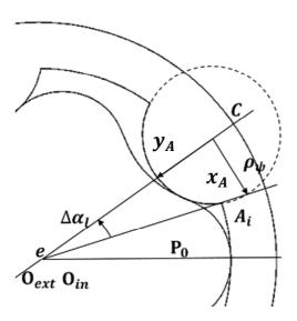
Figure 26: Determination of the circumferential length for radial ports
