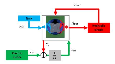
Figure 41: Interfacing the pump model with other components
