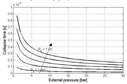
Figure 5: Example of cavitation bubbles collapse time
