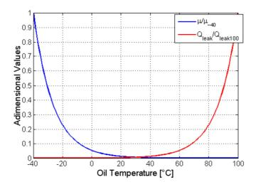
Figure 4: Viscosity and leakage behavior on oil temperature
