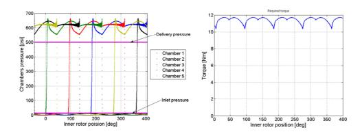
Figure 34: Fluid pressures (left) – simulated net torque (right)
