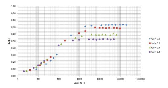
Figure 77: CFD results: discharge coefficient,  $\alpha = 30^{\circ}$
