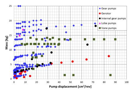
Figure 13: Catalogues data – pump's mass vs displacement
