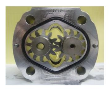
Figure 7: An external spur gears pump<sup>2</sup>
