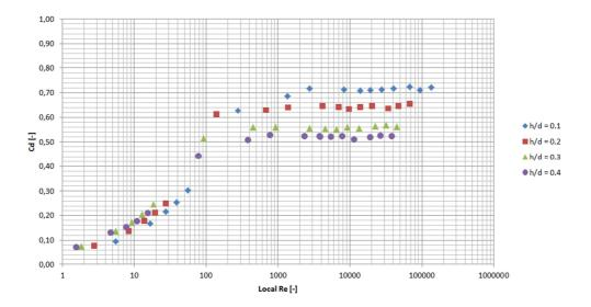
Figure 78: CFD results: discharge coefficient,  $\alpha = 45^{\circ}$
