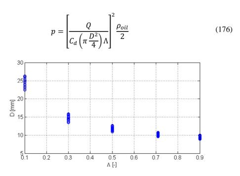
Figure 86: Inlet port diameter vs  $\Lambda$  - 45°
