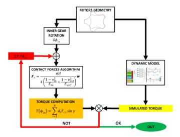
Figure 32: Algorithm for contact forces estimate
