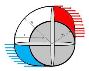
Figure 17: Unbalanced vane pump scheme
