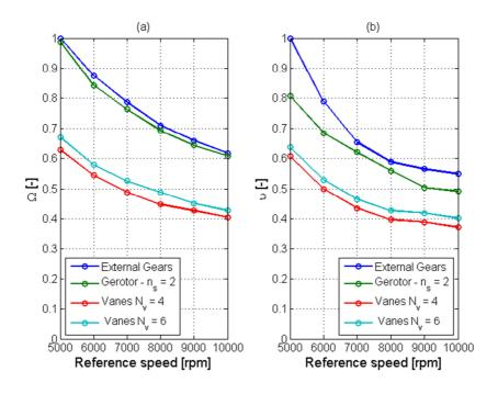
Figure 21: Mass (a) and envelope (b) comparison
