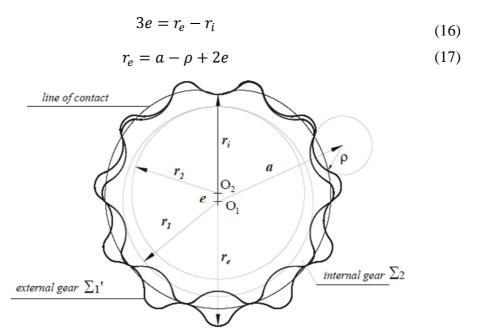
Figure 14: Geometrical parameters for epitrochoidal gerotor pumps
