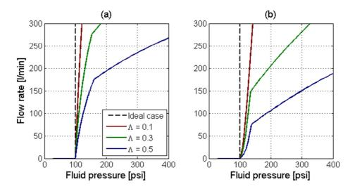
Figure 90: Valve characteristics: (a) 100 °C – (b) -40°C
