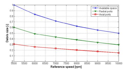
Figure 46: Maximum size of the expelled particles
