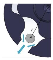
Figure 44: Spherical debris – radial ports
