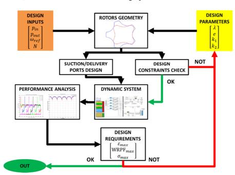
Figure 25: Design loop for gerotor pumps
