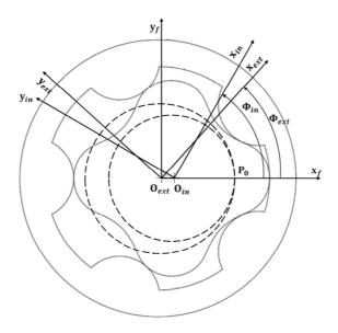
Figure 23: Reference systems for gerotor profile definition
