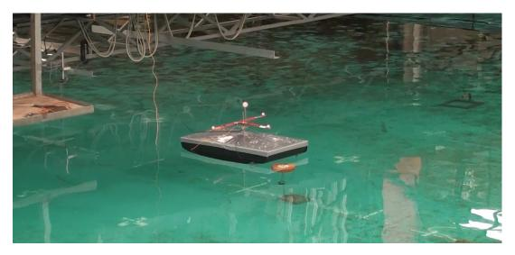
Figure 2.17 Hydrodynamics Tank Tests. Floater moored to the tank floor. 6 DOF analysis.
