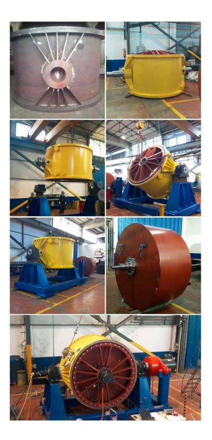
Figure 4.12 The gyroscope: assembly of the first unit.
