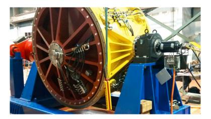
Figure 4.16 The gyroscope: flywheel lubricating system, oil recovery pump and rotary hydraulic joint.
