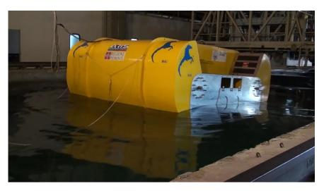
Figure 1.7 ISWEC prototype, 1:8 scale for Pantelleria site. Rome INSEAN wave tank.
