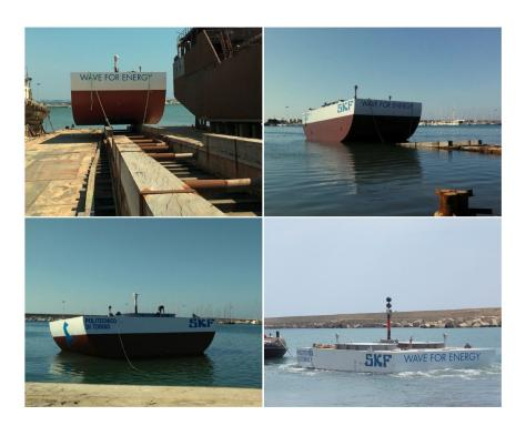
Figure 4.6 The floater: launch and ballast filling operations.
