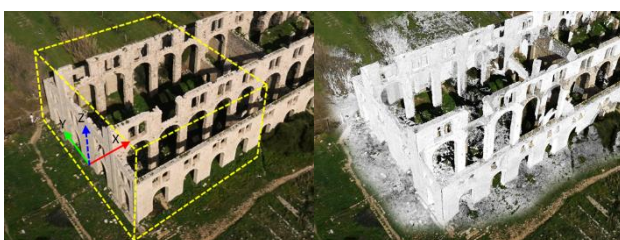
Figure 5. Test area for SBM2017: bounding box and XYZ local reference system (at left), TLS global cloud (at right).
