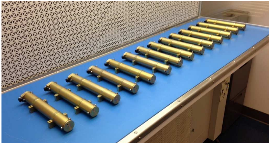
Figure 52 Magnetic torquer example: rod configuration
