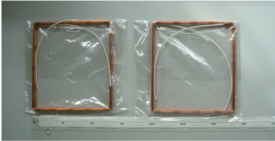
Figure 51 Magnetic torquer example: coil configuration
