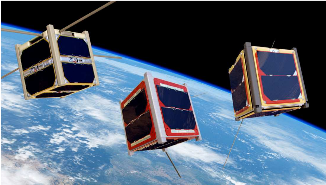
Figure 3 CubeSat spacecraft. The three winners of first ESA Fly Your Satellite! competition: OUFTI-1, e-st@r-II, AAUSAT-4. Credits ESA
